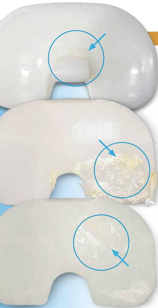
Typical wear associated with conventional polyethylene knee inserts.
